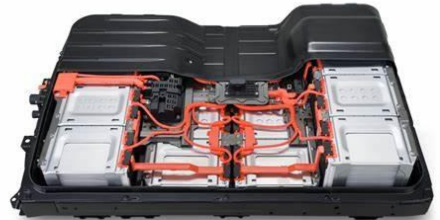
Nissan EV Battery Pack, with Modules Displayed, Source: Nissan
