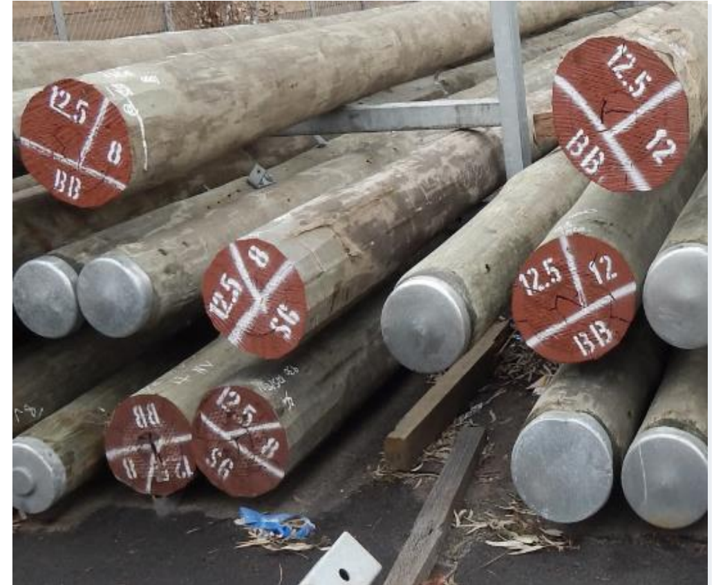
Size & Strength of Wood Poles (Metres/ kN)
